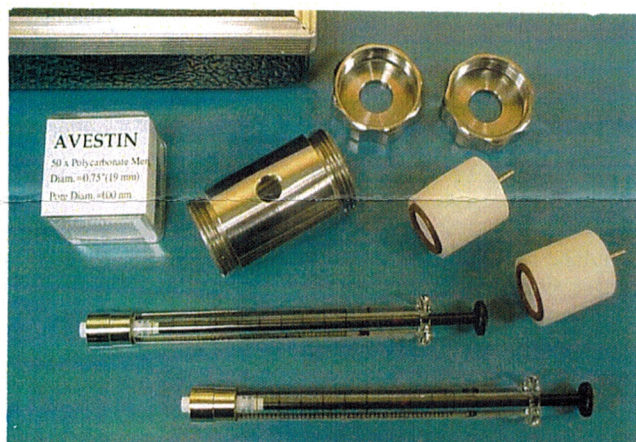
Figure 2: The LiposoFast-Basic consists of a stainless steel housing, membrane support, two 0.5mL syringes, and 50 polycarbonate membranes with 100nm pore diameter.
